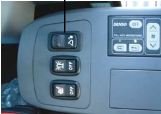
fig 3.22 Example of an OEM style on/off operating switch. (Switches differ with machine interior)
