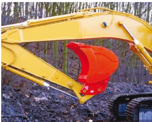
fig 2.3 Miller Scoop Bucket and Miller Coupler in transit mode
