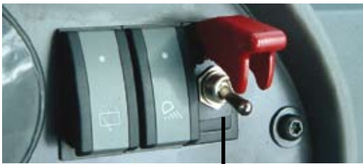
fig 3.23 Example of a Miller style on/off operating switch (switch style does differ)
