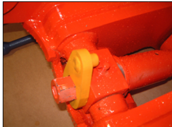
Once the coupler is firmly clamped onto the bucket/attachment pins, fit the locking cap as shown
