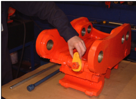
Once the coupler is firmly clamped onto the bucket/attachment pins, fit the locking cap as shown
